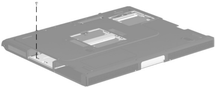
Figure C-8. Phillips M2.0 × 4.0 Screw Locations
